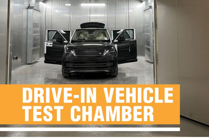
ETC's Drive-in Chambers simulate a wide range of environmental conditions and can include options such as heated road, solar, and velocity simulation.
